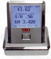
Black and Decker's Power Monitor (\$100; Blackand Decker.com) and the Energy Detective (below; from \$140; TheEnergyDetective.com) are two devices that will tell you exactly how much it costs per month and per year to run an appliance. In each, a sensor on your fuse box wirelessly transmits to a monitor with a LED readout that you can tote around the house; switch appliances off and on, and you can easily spot the cost.
